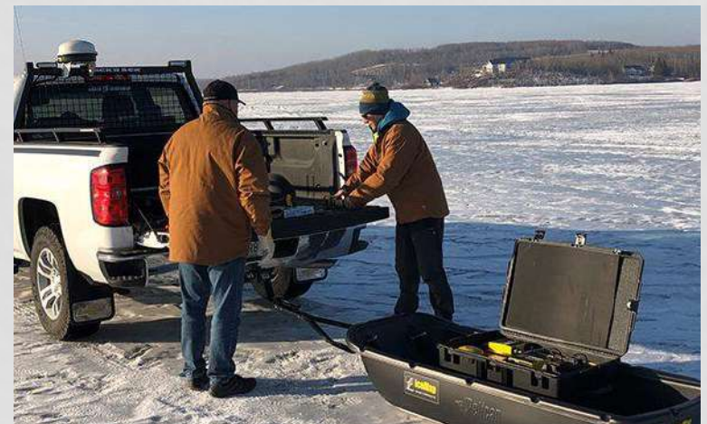
Measuring ice thickness using a radar system
