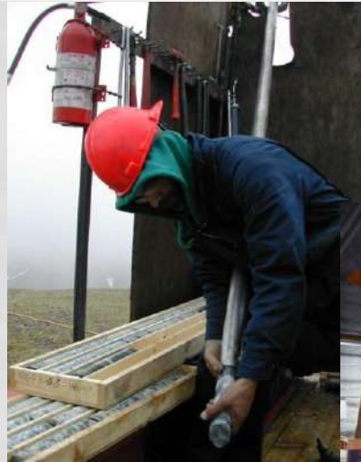
Winter drilling & Removing drill core from tube
